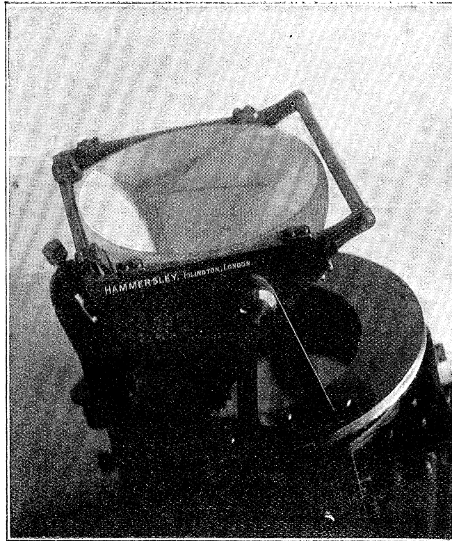
Details of prism mounting.
